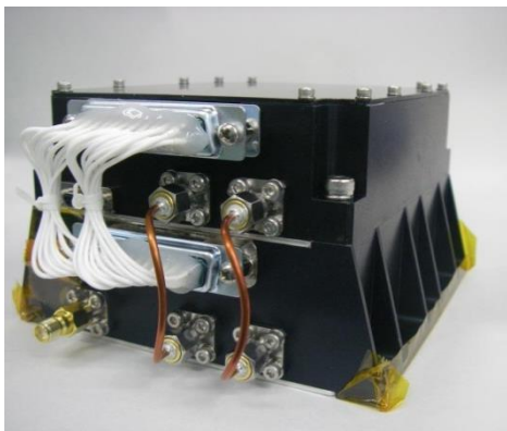
Fig. 2 Flight model of X band transmitter. DC power consumption is 22 W and mass is 1330 g.
