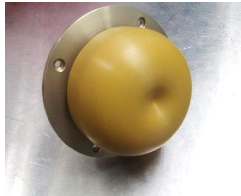
Fig. 6 Onboard iso flux antenna. Peak gain is 5 dBi and mass is 149 g.
