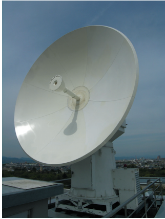
Fig. 7. S/X dual bands 3.8 m antenna. Peak gain of X band is 47.5 dBi.
