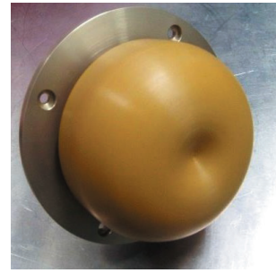
Fig. 6. Onboard iso flux antenna. Peak gain is 5 dBi and mass is 149 g.
