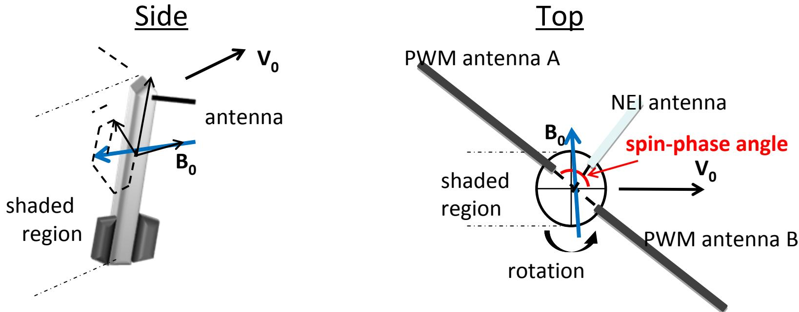
Fig. 7 Schematic side and top view of a moving rocket.
