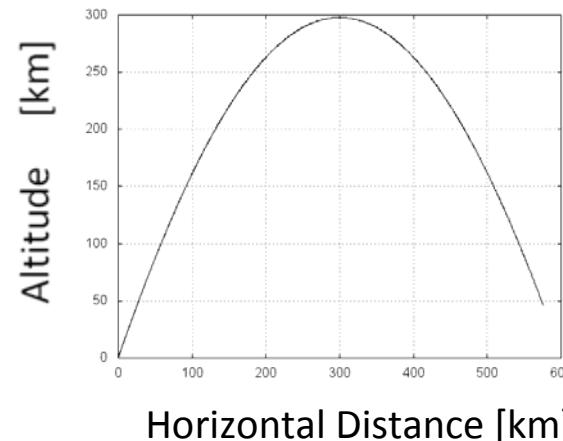
Fig. 4 Trajectory of the S-520-26 rocket.
