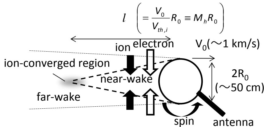
Fig. 2 Schematic picture of the wake.
