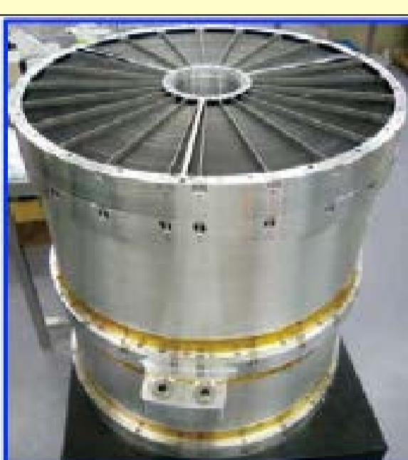
Half size (in diameter) of the ASTRO-H Hard X-ray Telescope(HXT; left panel). Focal Length will be 6m, 1/2 of the ASTRO-H.
