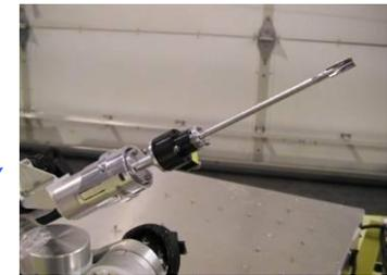
**Vane shear test tool**
