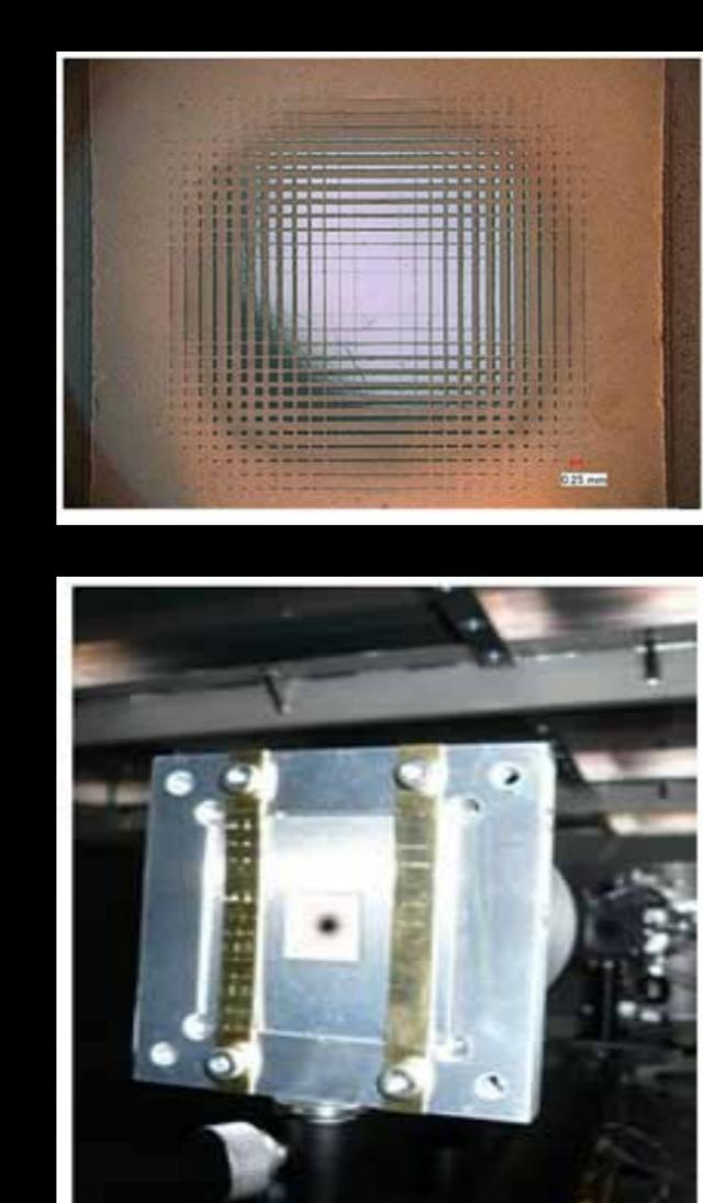
Left-top: fabricated free-standing mask (classical checkerboard design). Left-bottom: the free-standing mask installed in a testbed. Right: fabrication process of the free-standing mask (Haze 2012, Enya et al. 2012).
