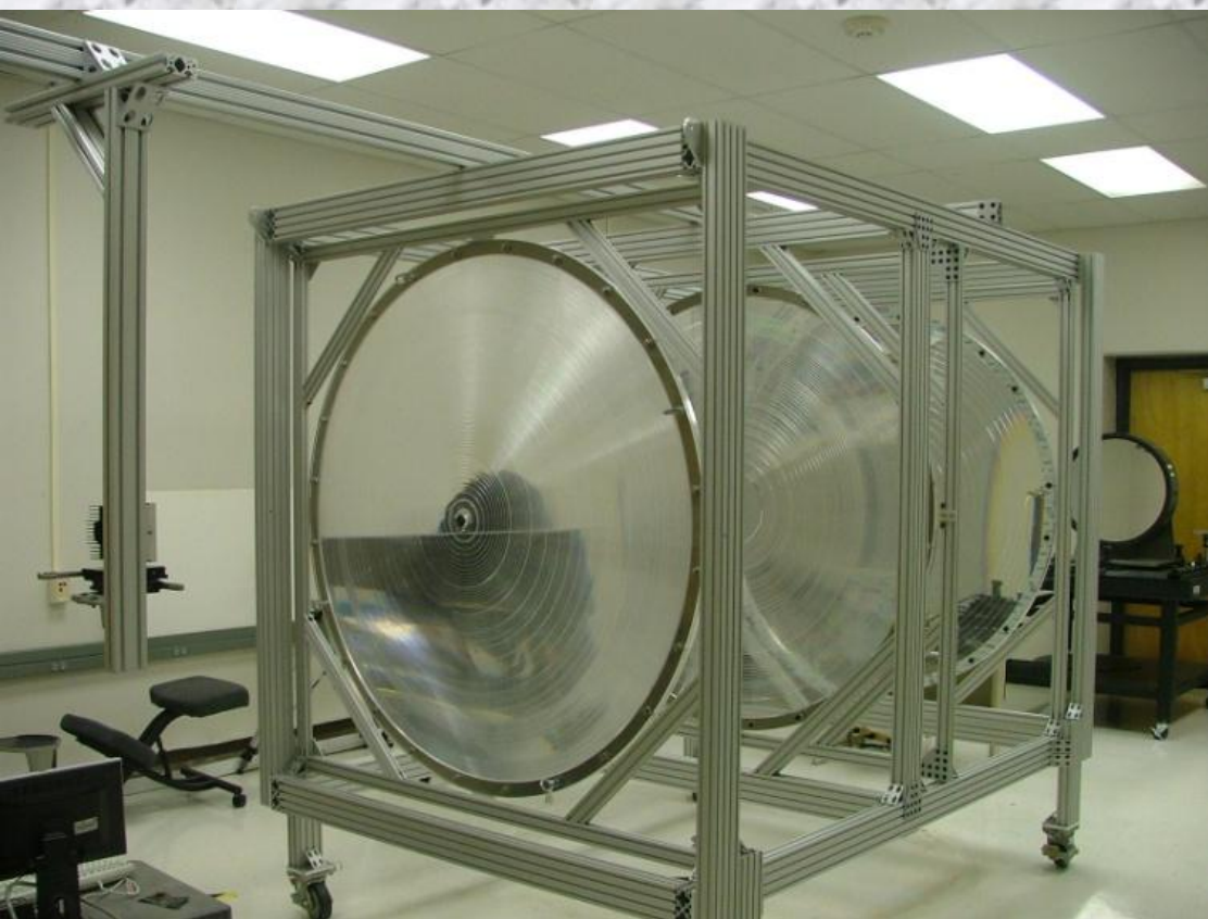
The prototype Lenses. These are the center part ( \phi 1.5\text{m} ) of the full lens system ( \phi 2.6\text{m} ).
