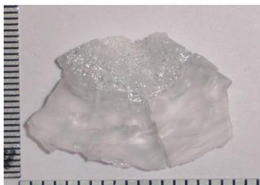
Fig.6 Spalled fragment
