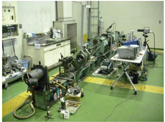
Fig.4 Two-stage light-gas gun installed at Hosei University.
