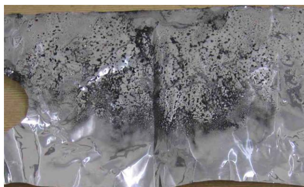
Fig. 8 deposited black soot on an aluminum sheet set on the inner wall of the pressurized chamber.
