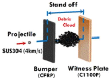
Fig. 1 Test configuration for fragment mass calculation.
