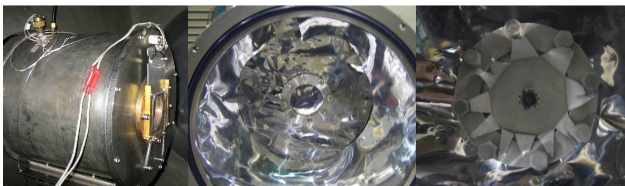
Fig. 3 Photographs of the pressurized chamber (left), the target and inside of the chamber (middle) and the target after an impact (right).
