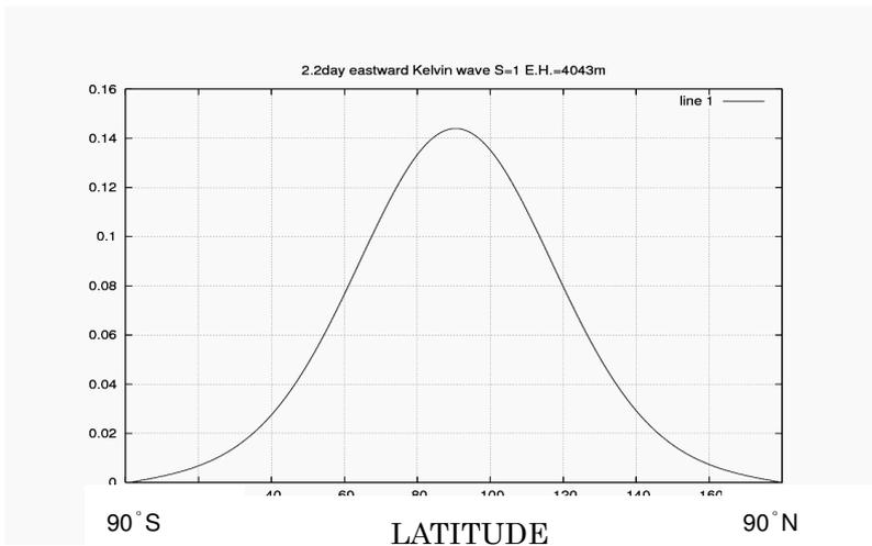
Figure (4): Kelvin wave solution of Laplace's tidal equation with 2.2day period eastward propagating mode.
