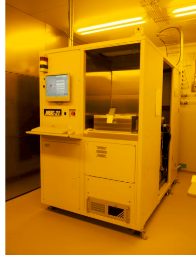
Fig. B.12 Conceptual diagram of the Bosch process (left), External view of DRIE (left)
