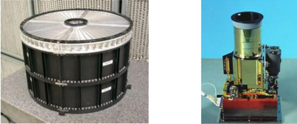
Figure 4.2 Photographs of the XRT (left) and the XIS (right) from the Suzaku Technical Description<sup>\*4.2</sup>.
