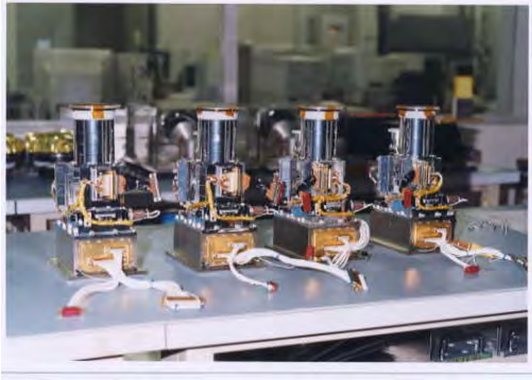
Figure 3.11: The four XIS detectors before installation onto Suzaku .
