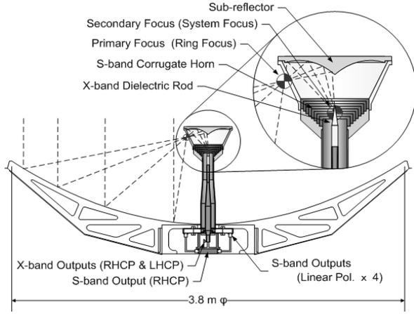
Fig.13 Structure of compact S/X dual band Cassegrain antenna with 3.8m diameter.
