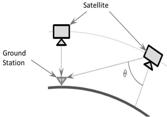
Fig.10 Iso-flux antenna with periphery - enhanced gain pattern compensates propagation loss at earth pointing mode.
