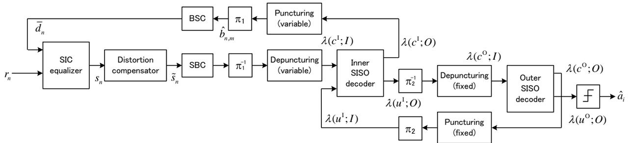
Fig.15 Block diagram of serially concatenated convolution turbo coding (SCCC) turbo equalizer at ground station. SIC: symbol interference canceller, SBC:symbol-binary converter, BSC:binary-symbol converter.
