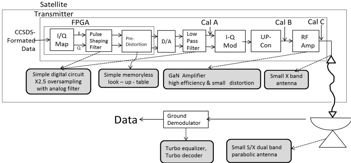
Fig.3 System block diagram of high-data-rate downlink. Several improvements are applied to satellite segment and ground segment.
