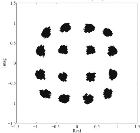
Fig.8 Measured IQ constellation of engineering model of transmitter with GaN HEMT amplifier of AB class. Symbol rate is 100Msps. RF output is 33dBm.
