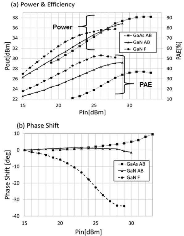
Fig.5 Comparison of three types of X-band RF power amplifiers. GaAs FET of AB class, GaN HEMT of AB class, and GaN HEMT of F class. (a) output power and power-added efficiency vs. input power. (b) phase shift vs. input power.
