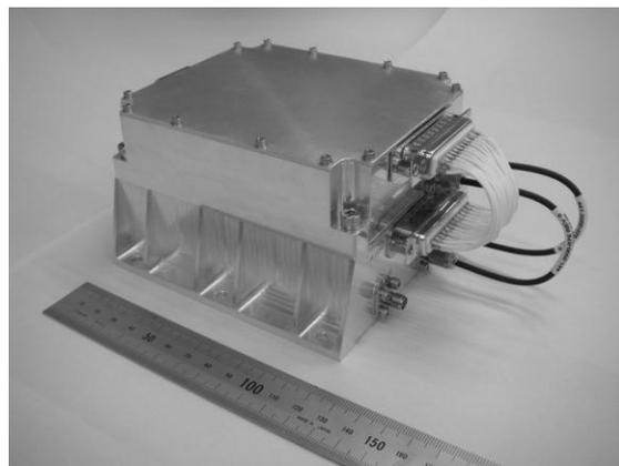
Fig.7 Photograph of engineering model of high-data-rate X-band 16QAM transmitter. Maximum data rate is 348 Mbps, RF output is 2W, DC power is 18W, and mass is 1330g and size is 120 x 120 x 73 mm<sup>3</sup>.
