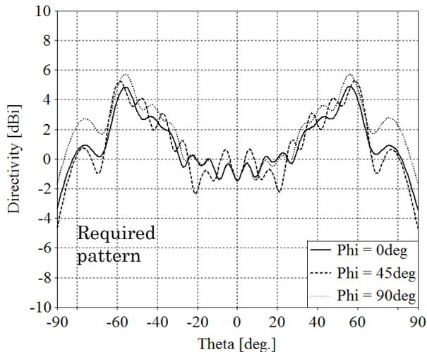
Fig.12 Simulation results of iso-flux antenna pattern with quadrafilary helix elements ( $\alpha=20^\circ$ ,  $D=10\text{mm}$ ,  $H=20\text{mm}$ ). Theta is angle from antenna normal plane. Phi is azimuthal angle. Required gain pattern is also plotted for 600km altitude.
