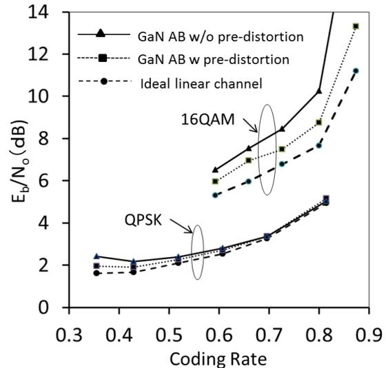
Fig.16 Simulation results of required  $E_b/N_0$  for 16QAM and QPSK as function of ACM coding rate. Broken line: ideal linear channel. Also  $E_b/N_0$  for GaN HEMT AB class amplifiers of 26 dBm input are shown. Solid line: without pre-distortion. Dotted line: with pre-distortion.
