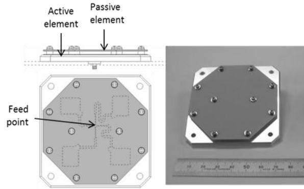
Fig.9 Structure and photograph of medium gain antenna with four active arrays and four passive arrays. Mass is 150g and size is 70 x 70 x 10mm<sup>3</sup>.
