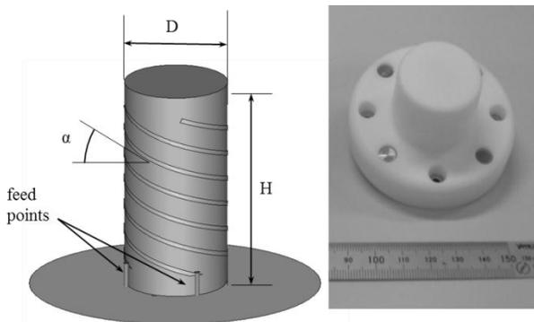
Fig.11 Structure and photograph of iso-flux antenna with quadrafilary helix elements. Mass is 150g,  $\alpha=20^\circ$ ,  $D=10\text{mm}$ ,  $H=20\text{mm}$ .
