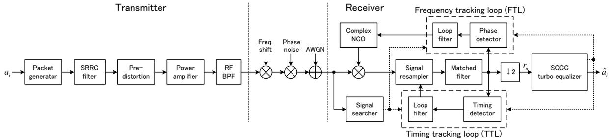
Fig.14 System block diagram of high-data-rate downlink including satellite segment (left) and ground station (right).
