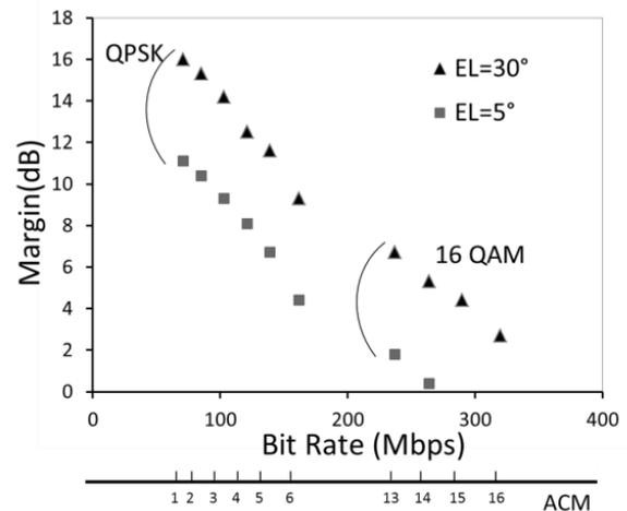
Fig.4 Link margin of high-data-rate down link as function of data bit rate or ACM number. Symbol rate is 100Mps, and elevation angle is 30° and 5° . Altitude is 600km and 13.5dBi MGA is applied. RF power amplifier is GaN HEMT of AB class with 26dBm input.
