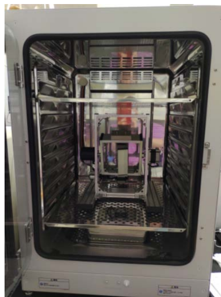
Fig. 1. 3D clinostat in CO 2 incubator.
