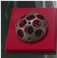
LRA(Laser Retroreflector Array) provided by NASA. The LRA consists of an array of multiple mirrors that are retroreflective and reflect light back in the direction of origin. Mass is approximately 21g.
