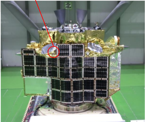
LRA(Laser Retroreflector Array) provided by NASA. The LRA consists of an array of multiple mirrors that are retroreflective and reflect light back in the direction of origin. Mass is approximately 21g.
