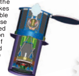
Structure of the Solar Optical Telescope installed on "Hinode"
