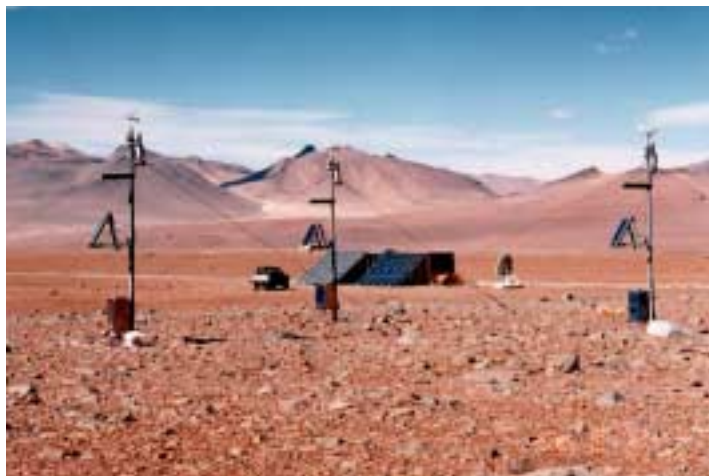
Fig. 5: Site testing instruments and containers at the 4800 m site of Pampa la Bola, Region II, Chile. Two containers equipped with solar panels and one of the antennas of the radio seeing monitor can be seen in the background. Three weather stations under cross calibration are seen in the foreground.
