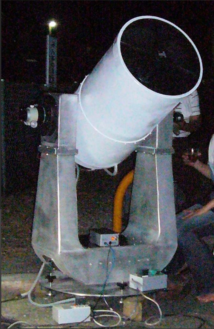
The new telescope in a test observation. It will be installed in the gondola upside down.
