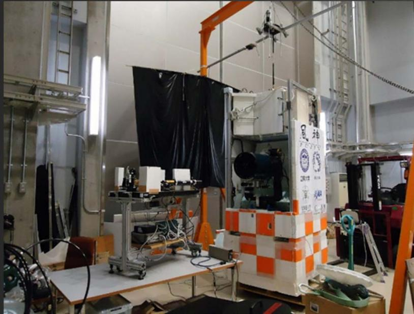
The gondola was hanged by a rope, which was rotated by a rotator as a perturbation generator. A laser was used as an artificial star light source of which the beam direction can be stirred by a vibrating mirror. Two parallel beams were introduced into the apertures of the telescope and star sensor.
