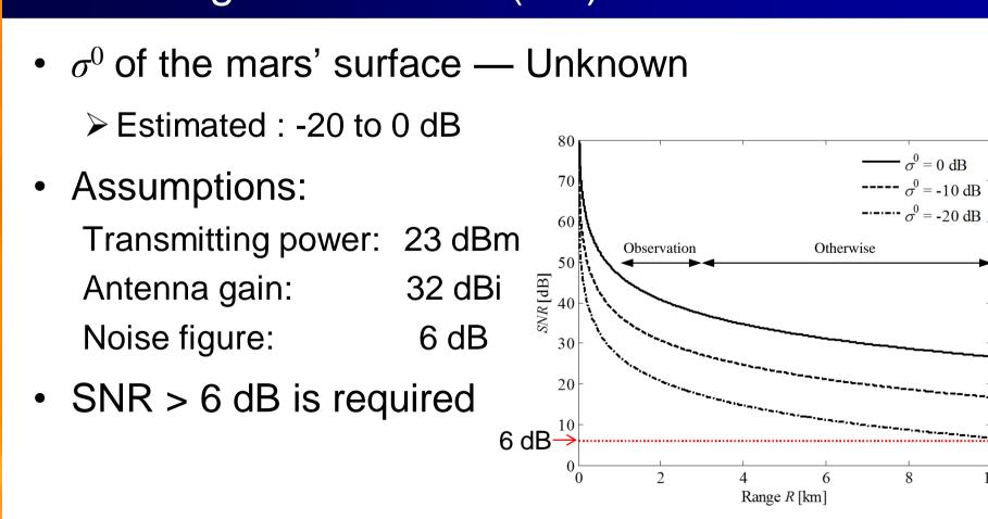
• The altitude can be measured when  $\sigma^0 = -20$  dB and R = 10 km (the worst condition).
