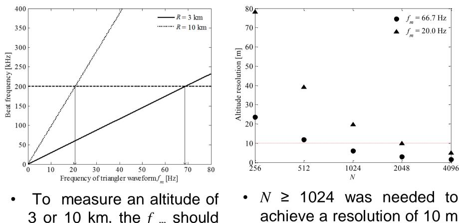
3 or 10 km, the  $f_m$  should be less than 20.0 or 66.7 Hz when the  $f_s = 400$  kS/s.
