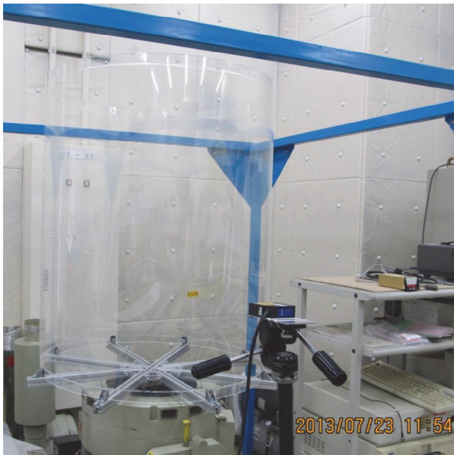
Fig.9 Vibration and buckling test of the large cylindrical shells.
