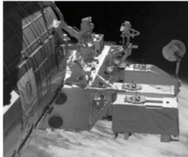
Figure 1. The SMILES instrument (the middle box to the right) aboard the JEM/ISS. Copyright NASA.
