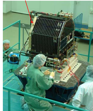
Antenna of Consert/Lander (Folded on the lander body)
