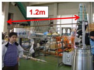
BeCu Ribbon Antenna (Sounding rockets) 伸長精度に難
