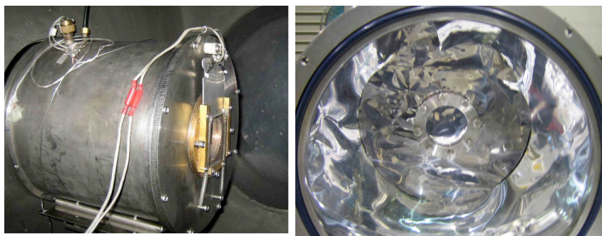
Fig. 1 Photographs of the pressurized impact chamber (left), and the target inside of the chamber (right).
