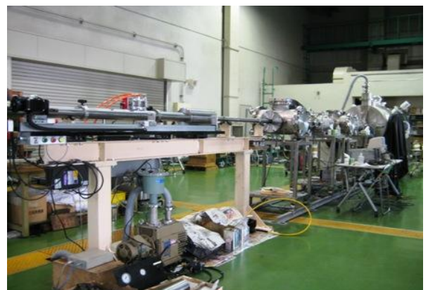
Fig.1 Photograph of two-stage light gas gun
