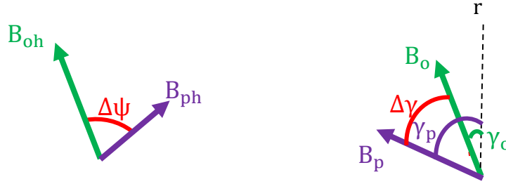
Figure 3.3 The relation of the directions of magnetic field and the shear angle. Left: \mathbf{B}_{oh} and \mathbf{B}_{ph} correspond to the horizontal component of observed and potential magnetic field respectively. Right: \mathbf{B}_o and \mathbf{B}_p correspond to the vector of observed and potential magnetic field respectively seen in the vertical plane.
