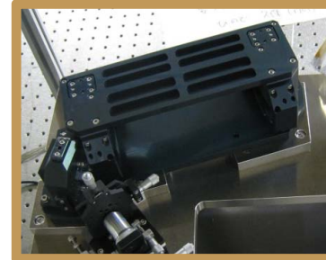
Slitjaw optics: mirror unit & filter unit
