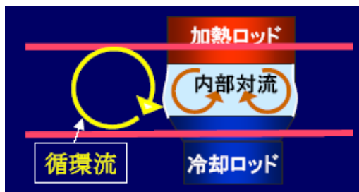
Fig.1 Partition disks to suppress the surrounding flow.
