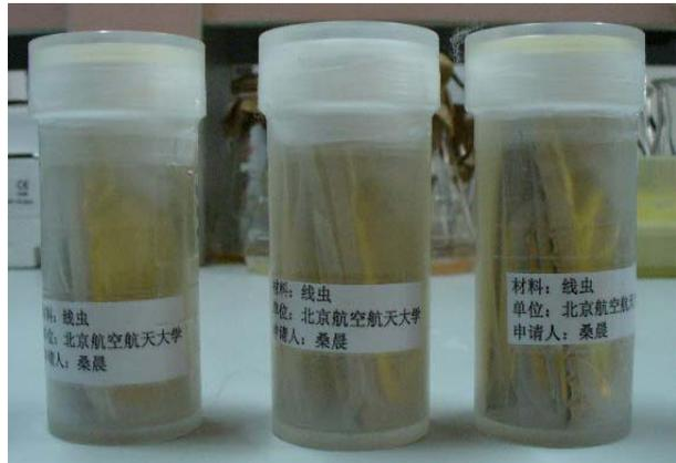
Fig.2 Plastic bottles used in this flight experiment. Five *C.elegans* culture bags were encapsulated in each bottle (see footnote below).
